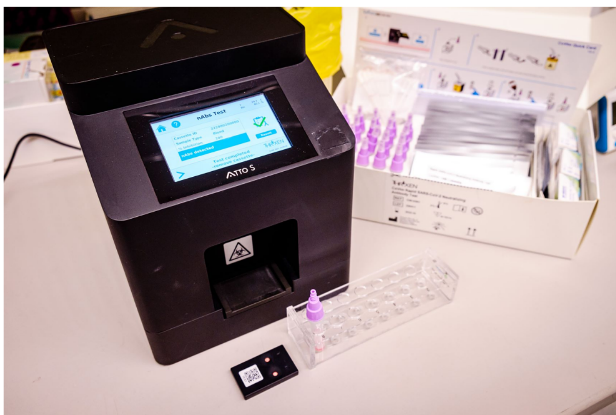
COVID-19 antibodies test kits (right) and the digital reader device (left in black), which can detect levels of COVID-19 antibodies from a drop of blood in just ten minutes.
